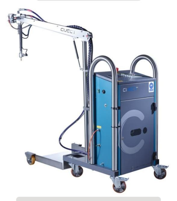
Ciject® One — RTM/VRTM Injection Machine
