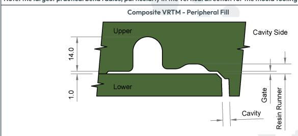
D seal groove to suit RD-20-0013 or RD-20-0011. Use RD-20-0010 (white) to form groove. Use RD-20-0016 (red) to form resin runner. Blend edge of groove R2 Typ.
