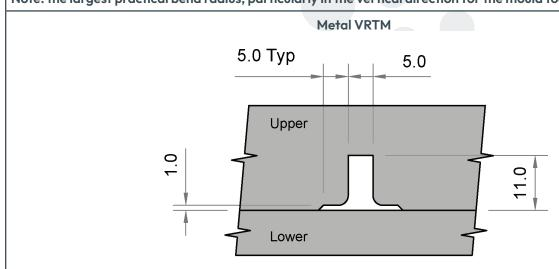
D seal groove to suit RD-20-0009. Runner detail varies on application. Blend edge of groove R2 Typ.
