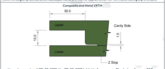
Lip seal groove to suit RD-20-0012. Use RD-20-0017 (white) to form groove. Blend edge of groove R2 Typ.
