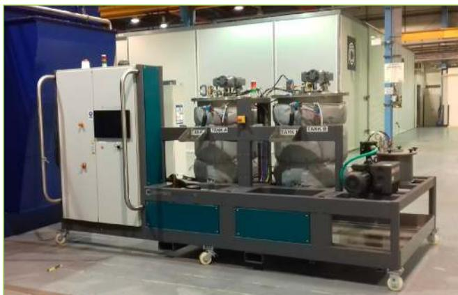
Fig. 2: Large Scale Resin Infusion (LSRI) equipment capable of injecting up to 400 kg of resin
